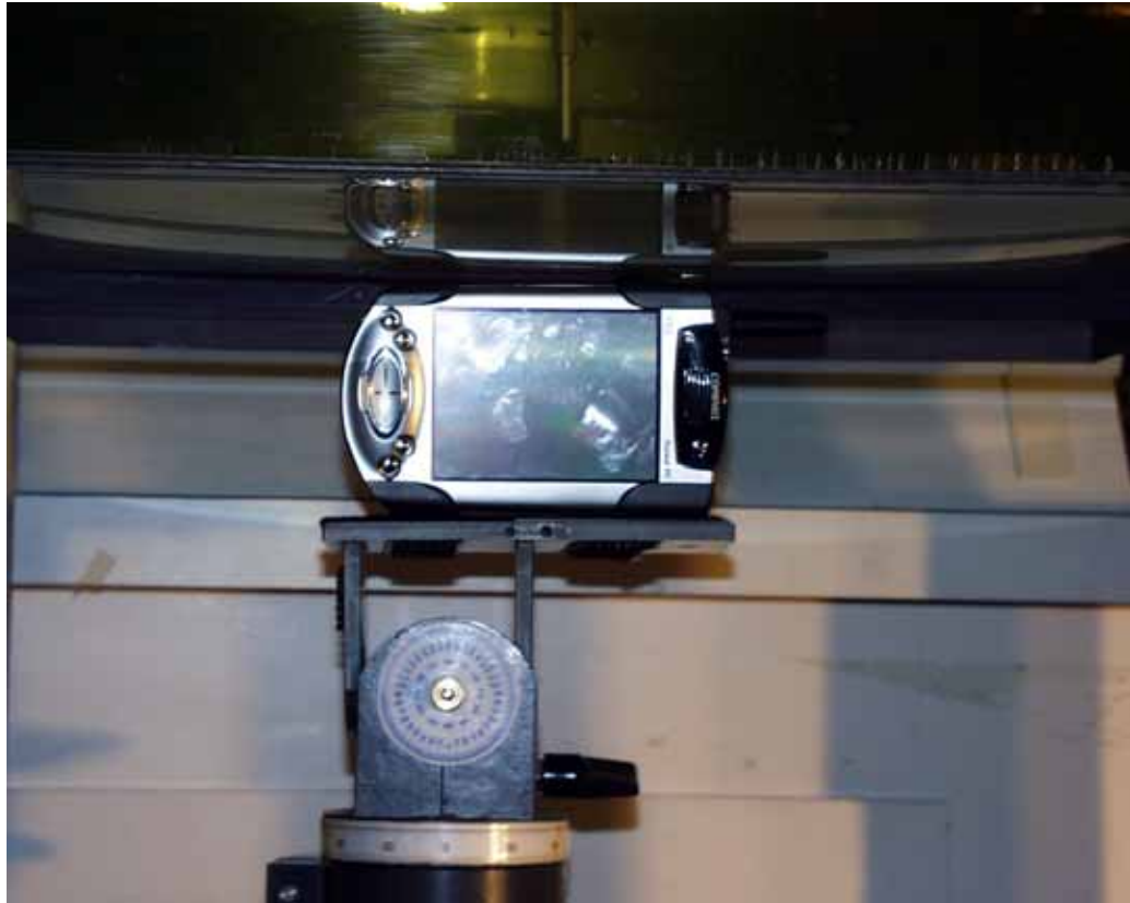
< Antenna side-face in parallel and in contact with the phantom >
