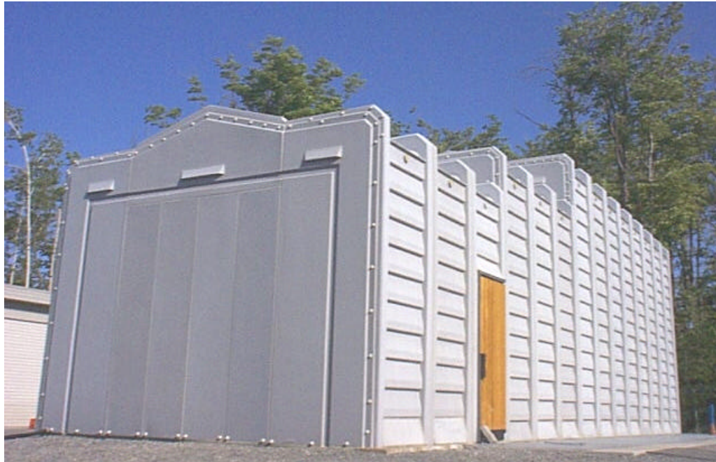
Fig. 1.b APREL's OATS (Open Area Test Site)
