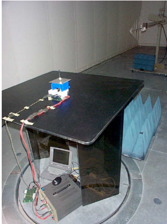
WaveNet BOOMER II tested for ERP
