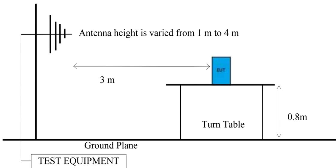
6.1.4. Fully Anechoic Chamber (3m) Setup Diagram for above 1GHz
