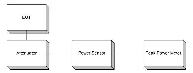
Minimum 6 dB Bandwidth Peak Power Spectral Density Spurious Emissions (conducted)
