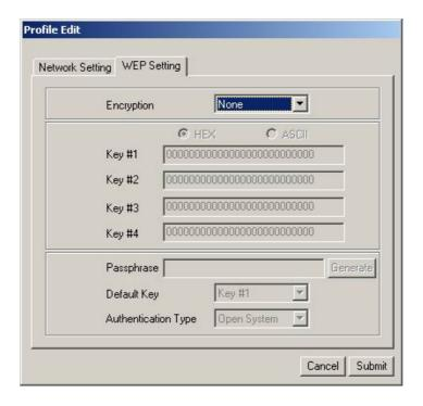
Additional security can be achieved by using the WEP (Wired Equivalent Privacy) encryption. WEP encrypts each frame transmitted from the radio, using one of the keys entered from this panel.
