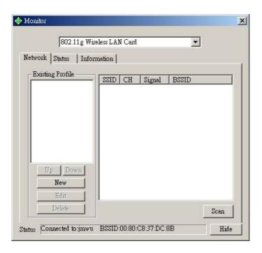
The screen at right shows all the Access Points or Adapters nearby when operating in Ad-Hoc mode. Click "**Scan**" to collect the SSID and Channel information of all the wireless devices near by.
