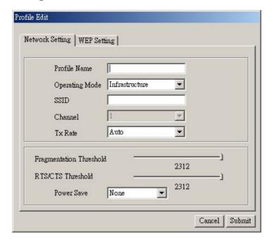
Click "New" in the Network page to set up the necessary parameters of the profile, and click "Submit" after the configuration has been changed.
