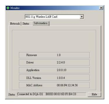
It shows the current *Firmware*, *Driver*, *Application*, *DLL Version and MAC Address* of the device.
