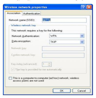
D. Click Authentication tab to select EAP type. (The EAP type should match the authentication server before access the authenticated network.)
