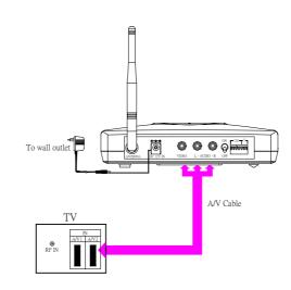
Note : If the accessory cable are euro/scart, they are different cable for transmitter and receiver. There has indicator on scart connector, please follow the indicator to install. For RCA cable they are identically.
