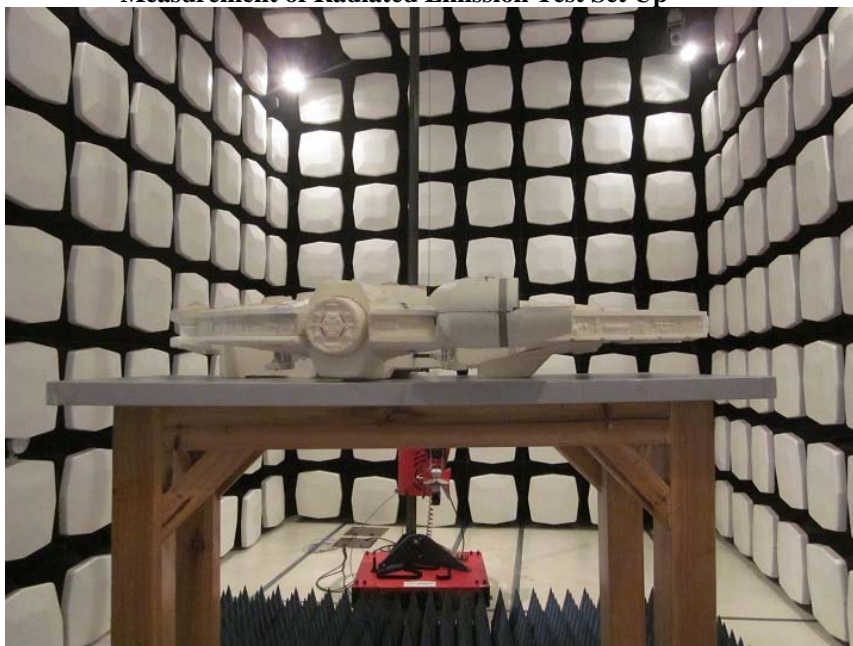
Measurement of Radiated Emission Test Set Up
