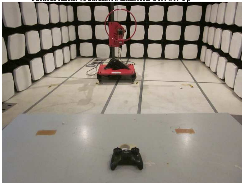
Measurement of Radiated Emission Test Set Up
