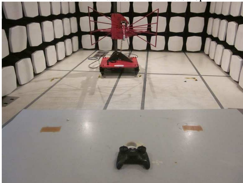
Measurement of Radiated Emission Test Set Up
