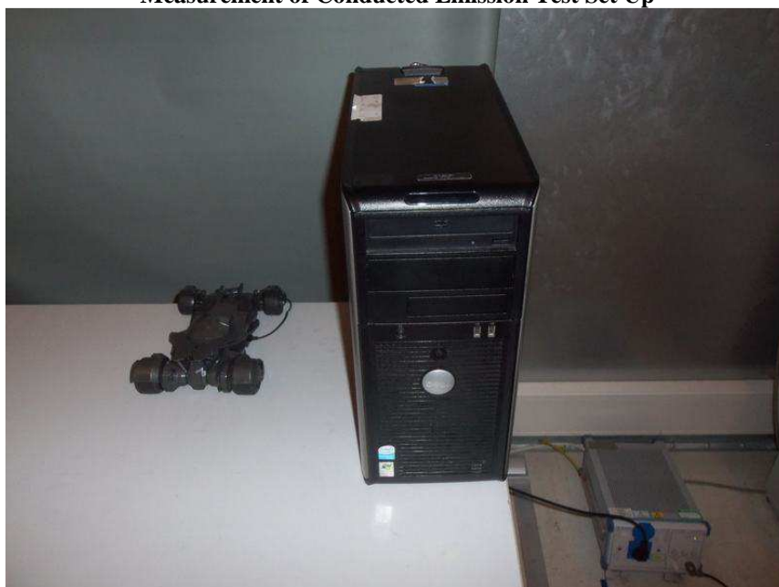
Measurement of Conducted Emission Test Set Up
