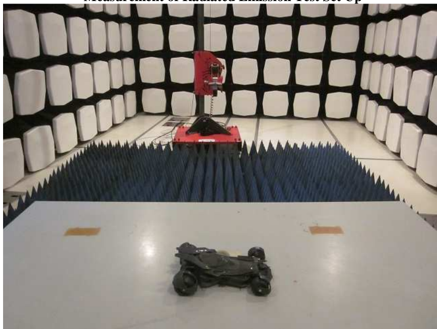
Measurement of Radiated Emission Test Set Up
