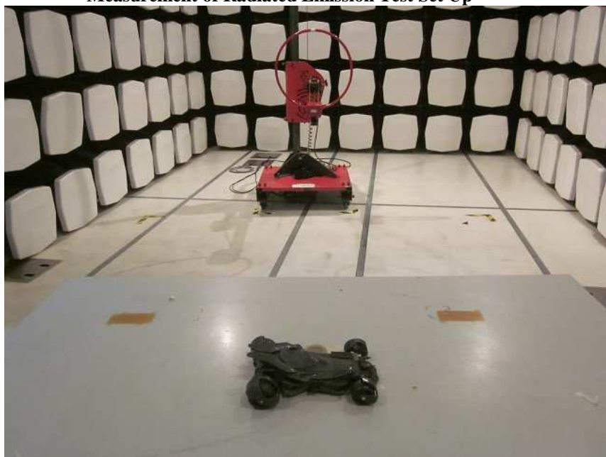
Measurement of Radiated Emission Test Set Up
