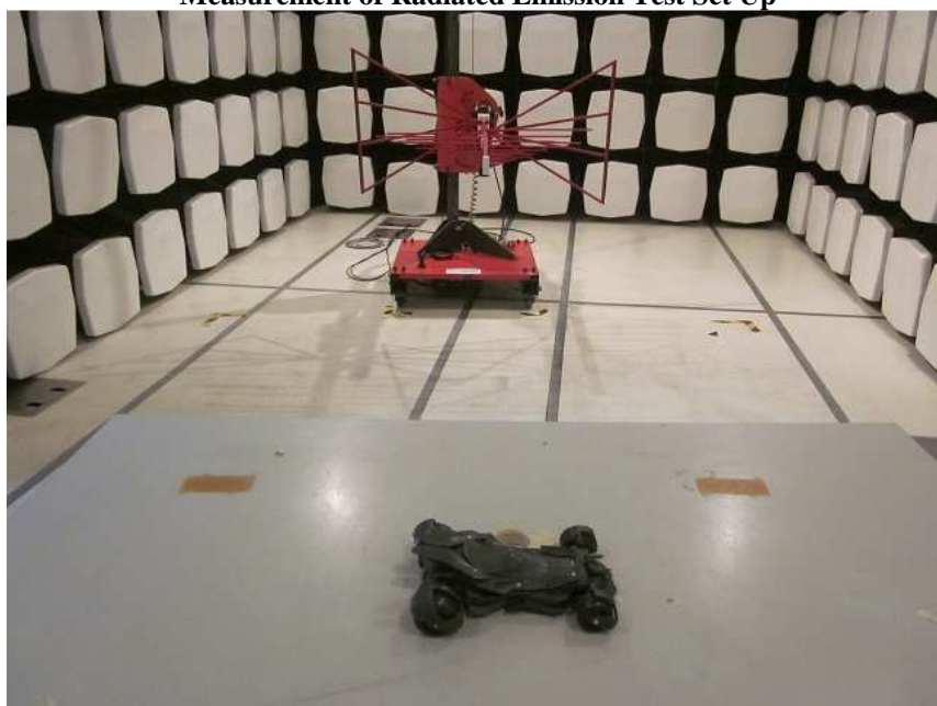
Measurement of Radiated Emission Test Set Up
