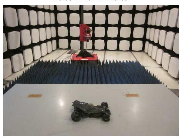
MEASUREMENT OF CONDUCTED EMISSION TEST SET UP
