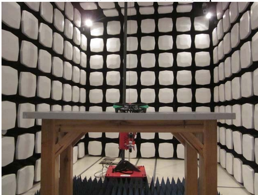
Measurement of Radiated Emission Test Set Up
