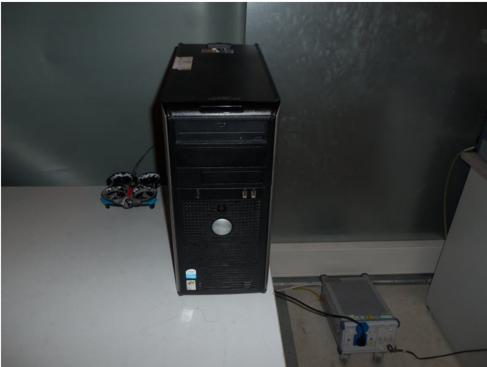
Measurement of Conducted Emission Test Set Up
