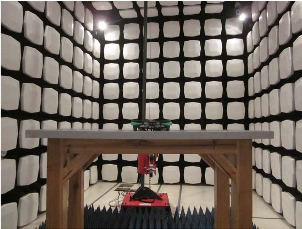
Measurement of Radiated Emission Test Set Up
