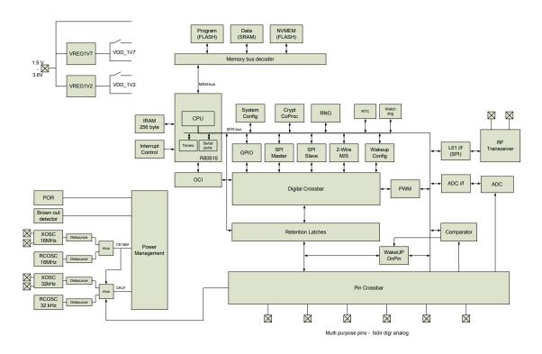
Figure 1. nRF24LE1 block diagram
