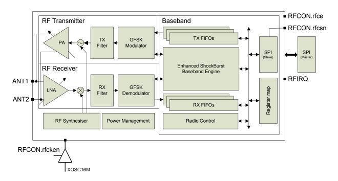
Figure 5. RF Transceiver block diagram
