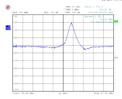
Bandedge Plot – Pursuant to FCC Part 15 Section 15. <u>227</u> Requirement (Pass)
