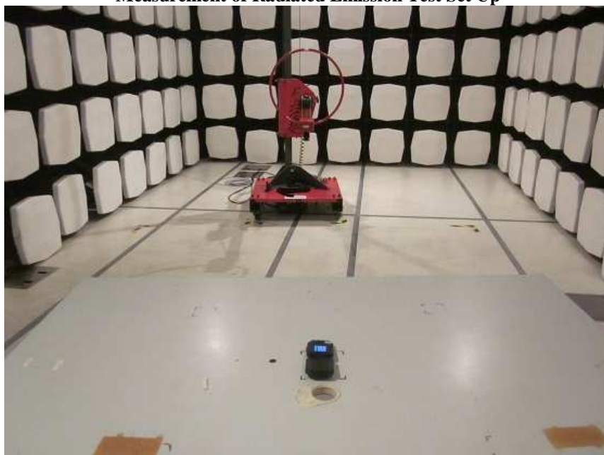
Measurement of Radiated Emission Test Set Up
