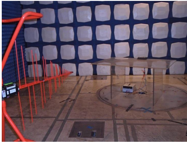
Photograph 1. Radiated Spurious Emissions, Test Setup, 30 MHz – 1 GHz
