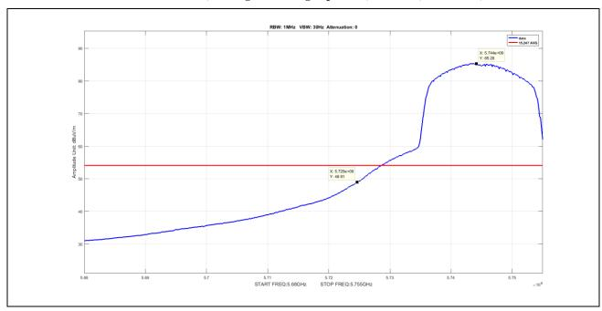
Plot 34. Undesirable Emissions, Average Band Edge Spurious, BW 20M, Ch 5745M, N Mode Port 2
