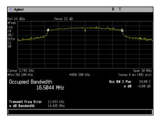
Plot 105. 6 dB Occupied Bandwidth, BW 20M, Ch 5745M, A Mode Port 1
