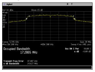
Plot 106. 6 dB Occupied Bandwidth, BW 20M, Ch 5745M, A Mode Port 2
