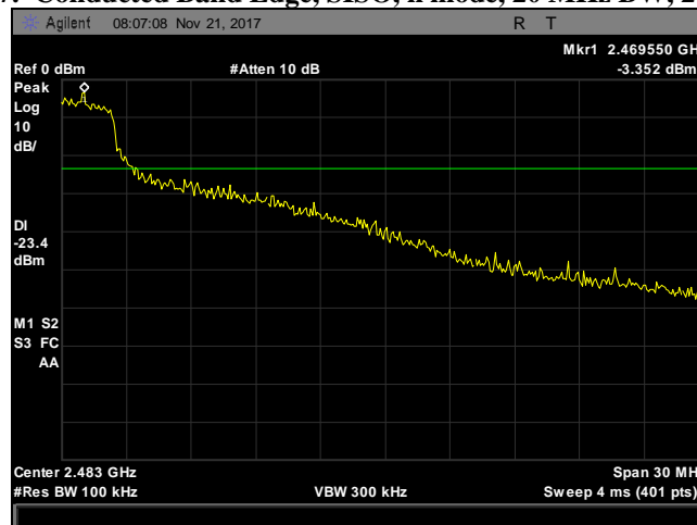
Plot 138. Conducted Band Edge, SISO, n mode, 20 MHz BW, 2462 MHz
