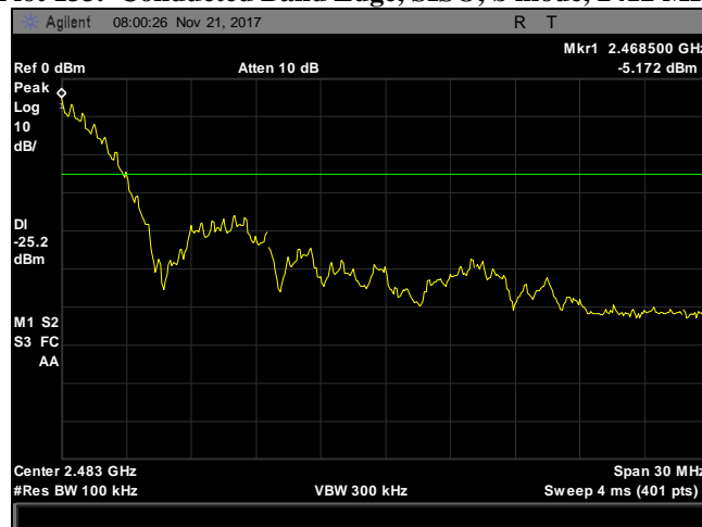
Plot 134. Conducted Band Edge, SISO, b mode, 2462 MHz
