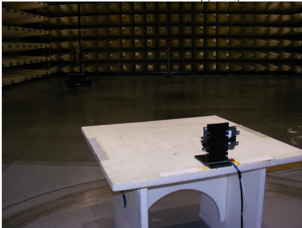
Photo 2: Radiated emissions test setup (> 1GHz)
