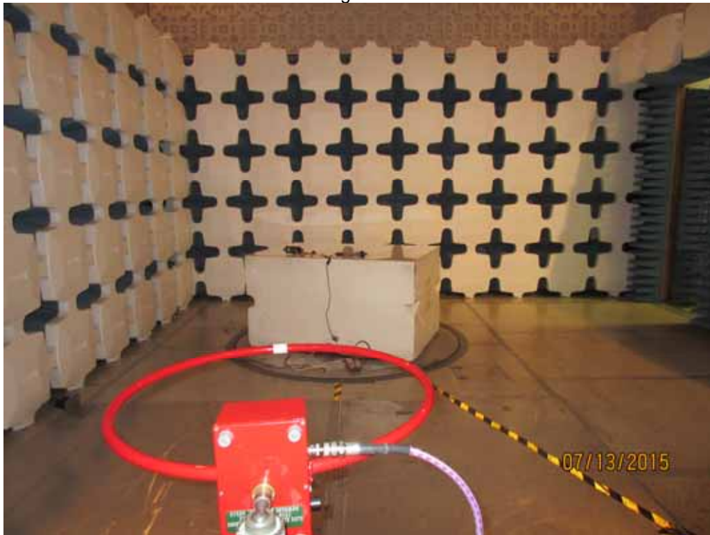
Test Setup for Radiated Emissions, 150kHz to 30MHz – Horizontal Polarization
