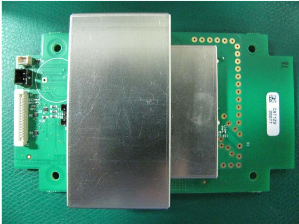
Figure 3 – Circuit Board with Shield, top side
