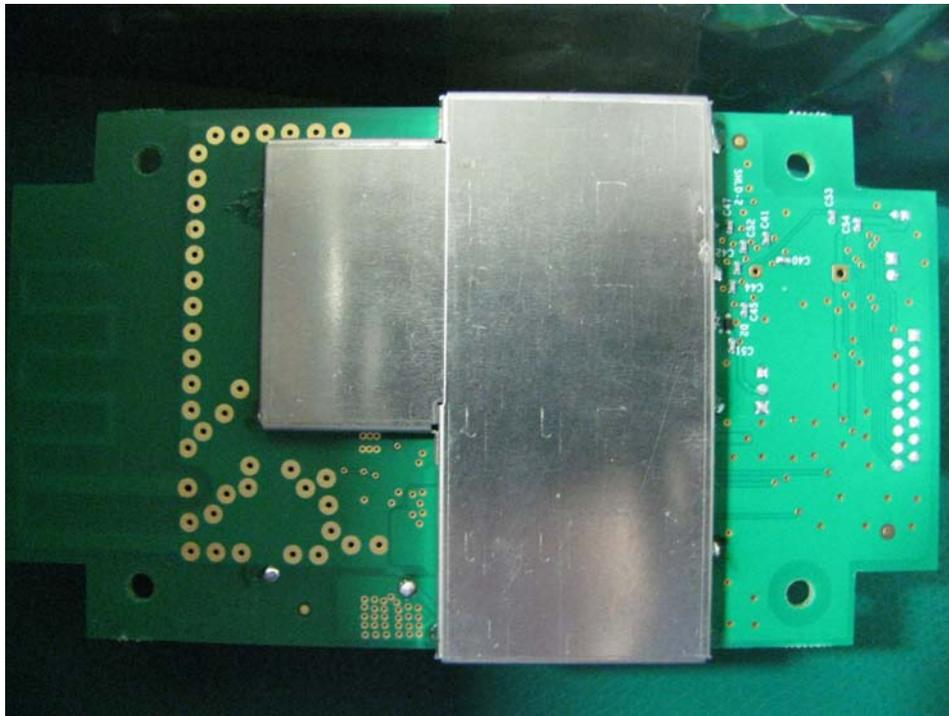
Figure 4 – Circuit Board with Shield, back side
