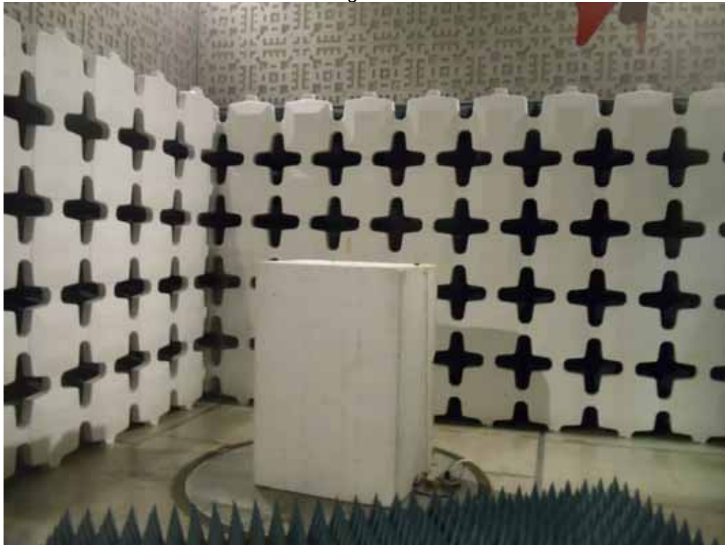
Test Setup for Radiated Emissions – 1GHz to 18GHz, Horizontal Polarization
