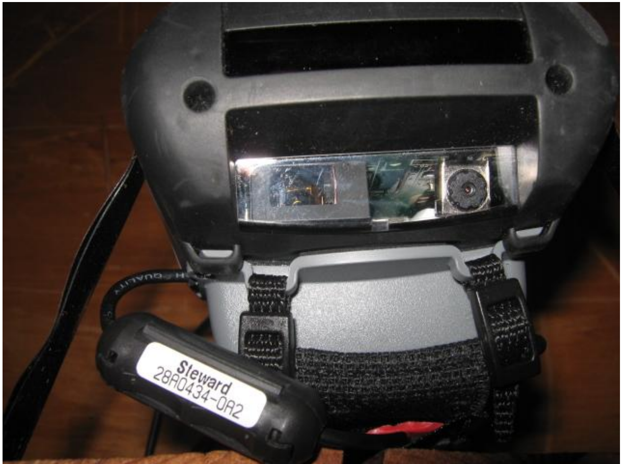
Figure 2: Ferrite bead used for radiated emissions
