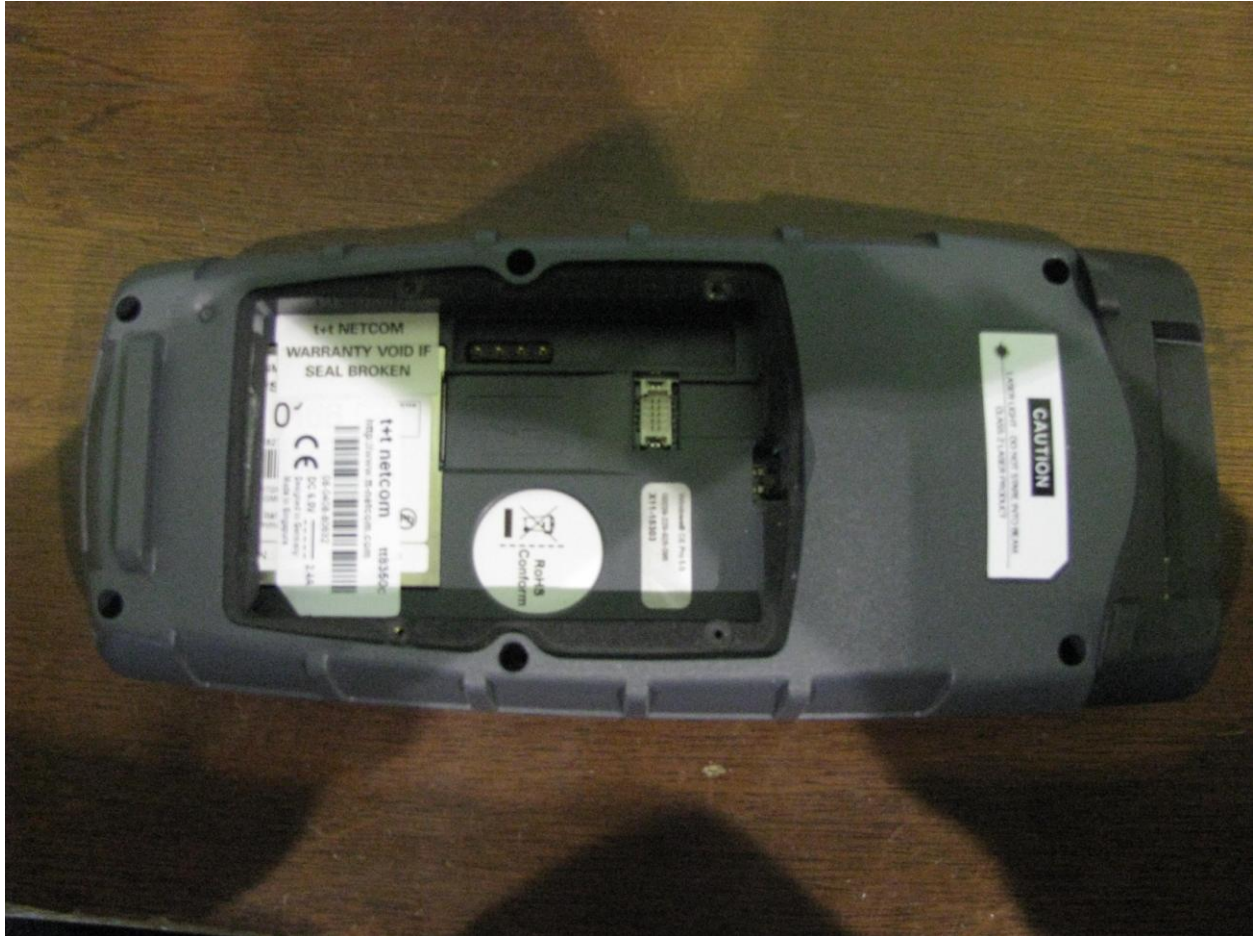
Figure 5: EUT Battery and RF module removed
