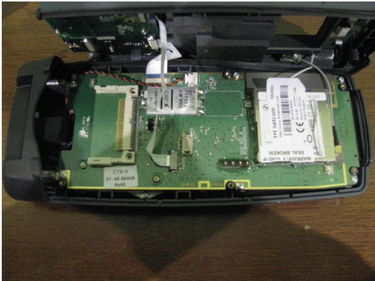
Figure 6: Back cover open (Top side of PCB)
