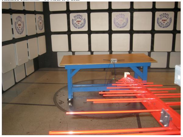
Note: In accordance with ANSI C63.4:2009 Section 6.2.2.1 and 6.2.2.2 the RS-485 and Ethernet auxiliary devices were remotely located from the test site.
