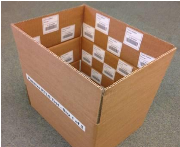
Figure 12. Unfolded carton with passive test tags.
