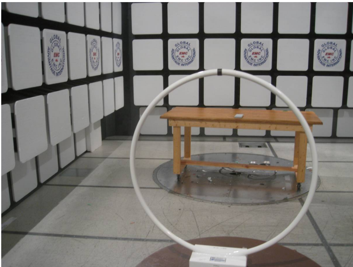
Radiated Emissions – 9 kHz to 30 MHz setup
