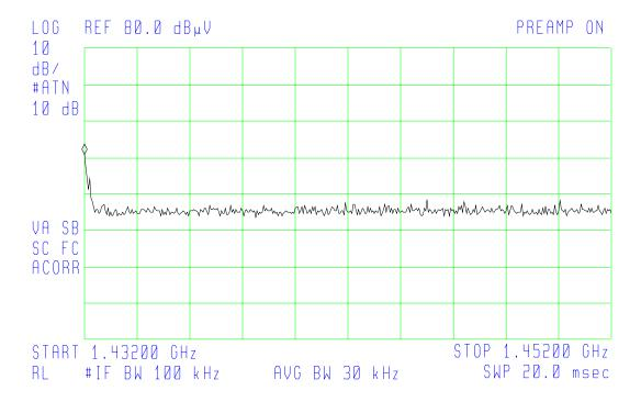
Plot shows upper band edge on left and 20 MHz window. A peak measurement of 50.61 dBuV/m with a limit of 54 dBuV/m avg, data shows a margin of 3.39 dB.
