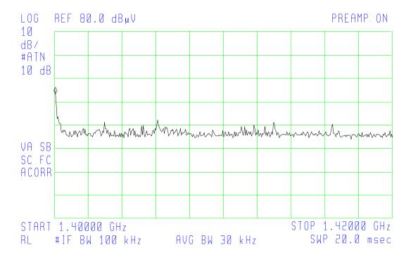
Plot shows upper band edge on left and 20 MHz window. A peak measurement of 53.34 dBuV/m peak, 33.34 dBuV/m Avg with a limit of 54 dBuV/m avg, data shows a margin of 20.66 dB.
