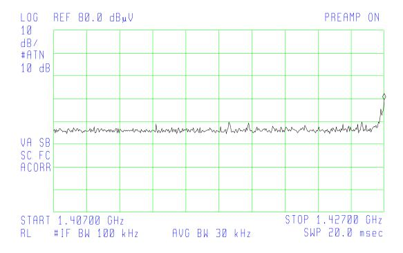
Plot shows lower band edge on right and 20 MHz window. A peak measurement of 49.40 dBuV/m with a limit of 54 dBuV/m avg, data shows a margin of 4.60 dB.
