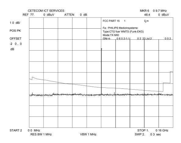
This plot shows peak values and the limit according to FCC15.209 at 10m distance. We made additional measurements with CISPR QP Detector and recalculated the results to 3m distance by adding 10.5 dB.
