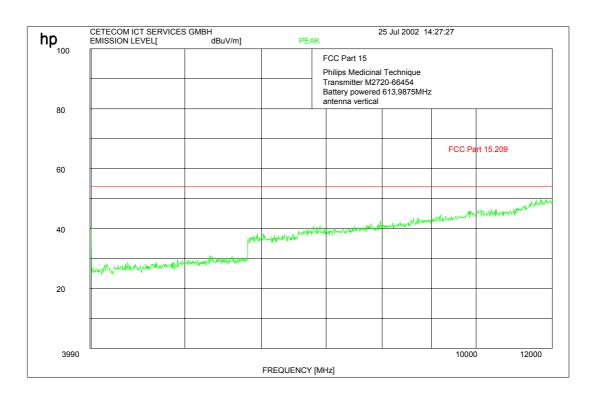
This plot shows peak values and the limit according to FCC15.209 at 3m distance. We made additional measurements with AV Detector.
