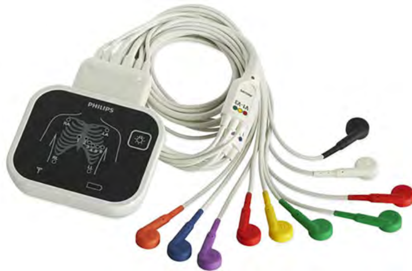
Figure 3-7 Wireless PIM and Lead Set
