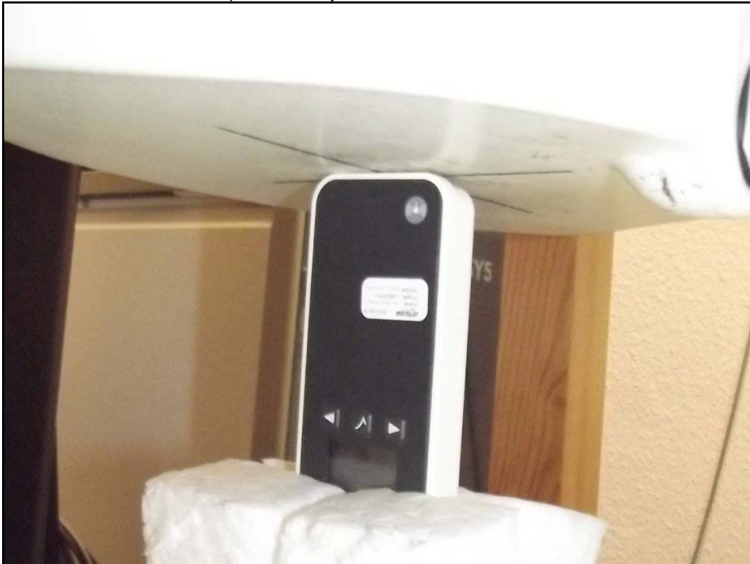
Photo 11: Test position body worn bottom side with 0 mm distance
