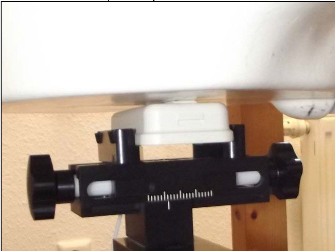
Photo 10: Test position body worn rear side with 0 mm distance
