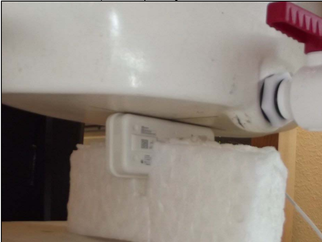
Photo 10: Test position body worn rear side with 0 mm distance
