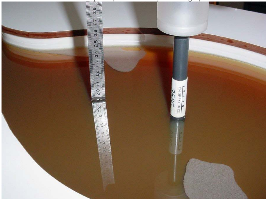
Photo 2: Liquid depth 5 GHz body simulating liquid
