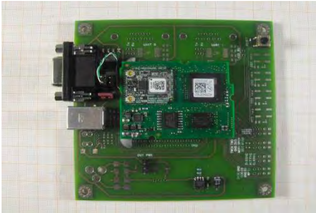
Photo 1: Interface board with test board and EUT
