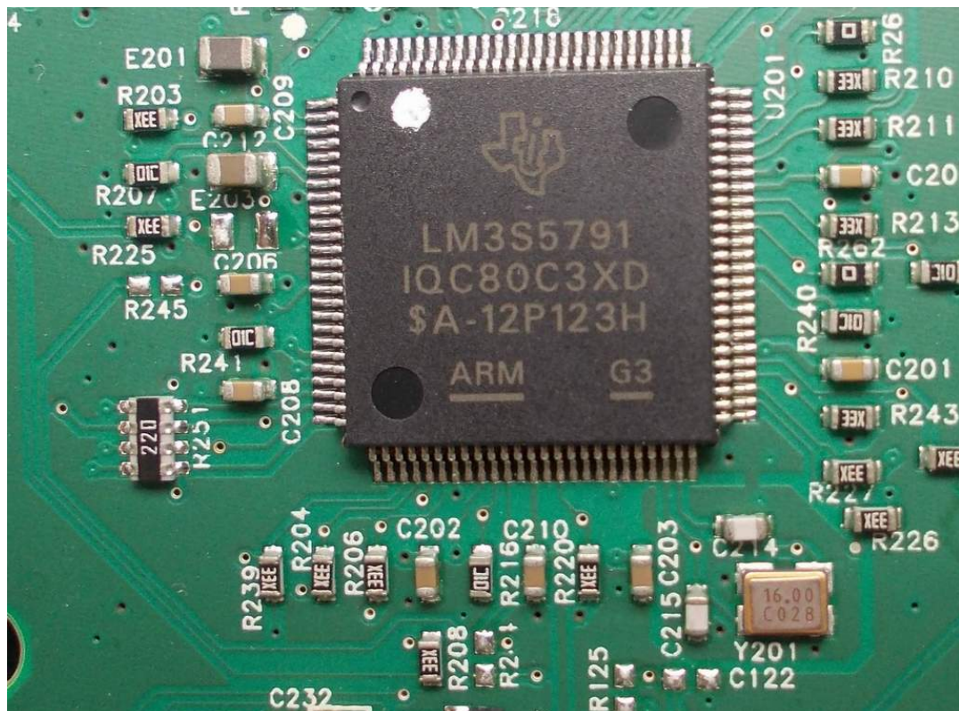
FIGURE 5 ADVANCED INTERFACE MODULE (M/N: ST801 AIM) CHIP & CRYSTAL #2 ON MAIN BOARD
