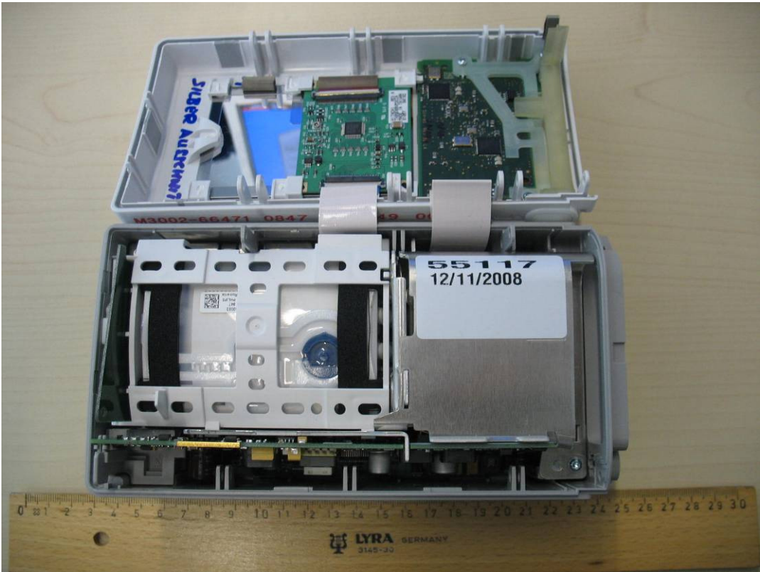
Photo 10: SRR Module in IntelliVue X2 Host Monitor
