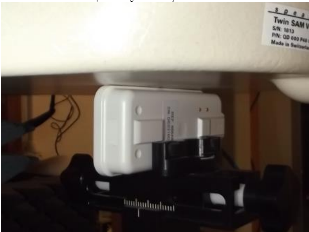
Photo 8: Test position right side body worn with 0 mm distance
