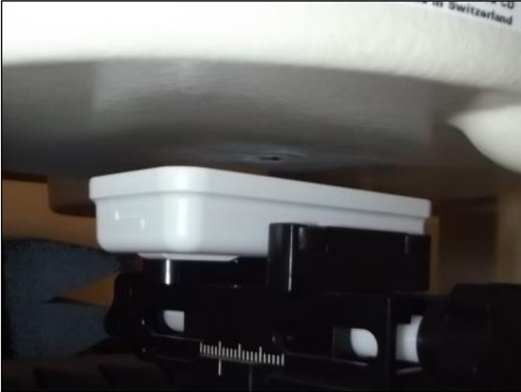
Photo 6: Test position rear side body worn with 0 mm distance
