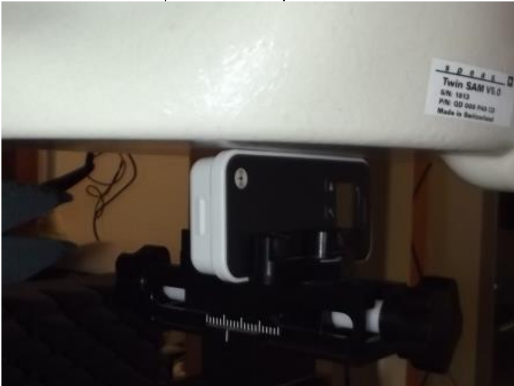
Photo 8: Test position right side body worn with 0 mm distance
