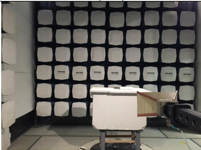
Radiated Emissions (>1GHz) – Front View
