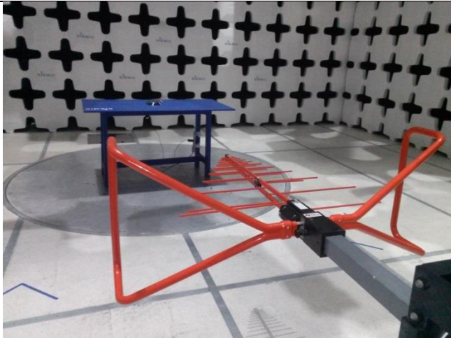
Radiated Emissions (<1GHz) – Front View
