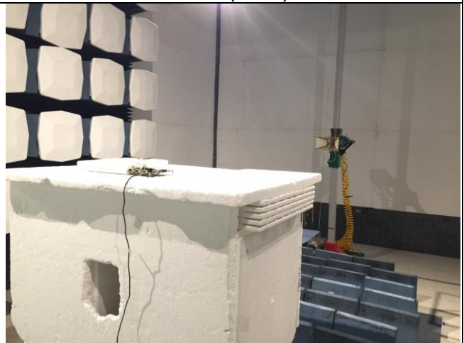
Radiated Emissions (>1GHz) – Rear View
