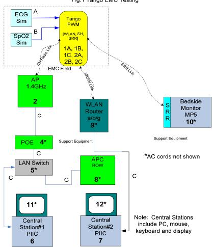
Note: Blk Diag #'s 2, 4, 5, 6 and 11 were configured as support equipment for this test.
