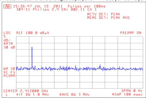
7.10.2 Determination of time averaged output power – Pulse width = 225  $\mu$ s.
