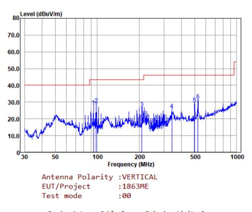
Test Mode: 00; Polarity: Vertical
