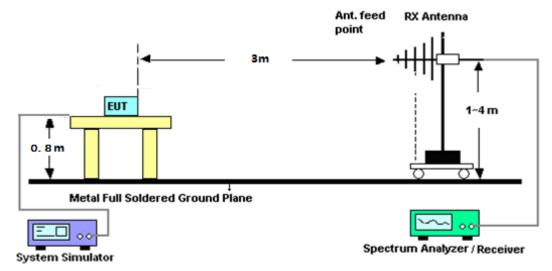
For radiated test from above 1GHz
