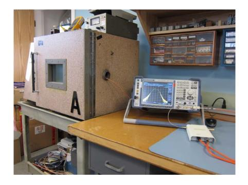
8.9. ERP Measurement - Close-up of Setup
