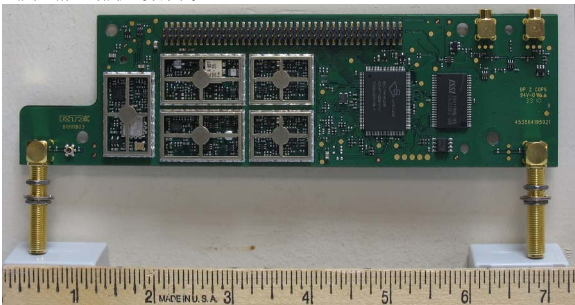
Transmitter Board – Covers Off
