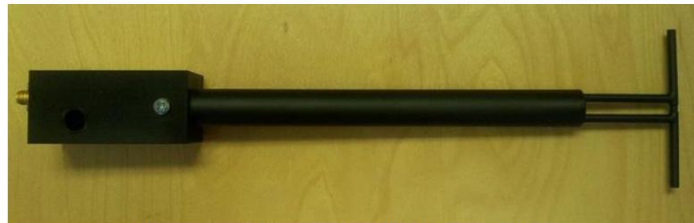
Figure 1 – MVG COMOSAR Validation Dipole
