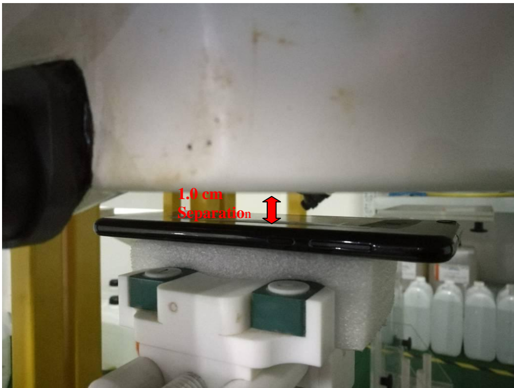
Body Setup Photo (LCD DOWN)
