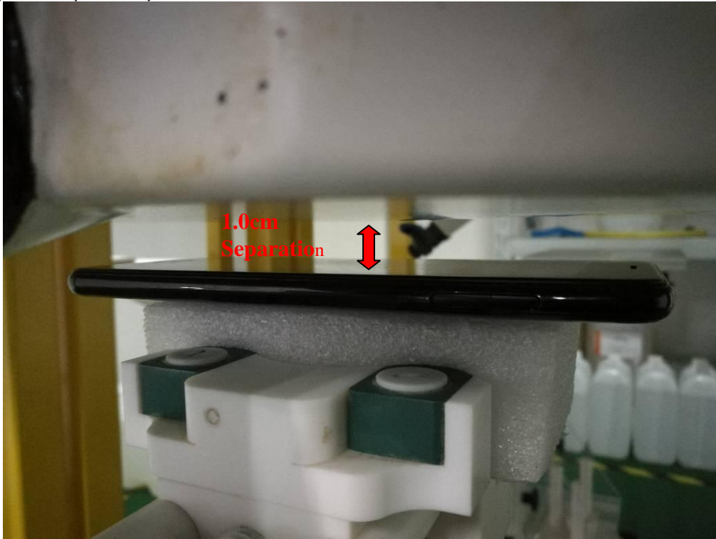
Body Setup Photo (LCD DOWN)
