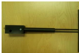
Figure 1 – MVG COMOSAR Validation Dipole
