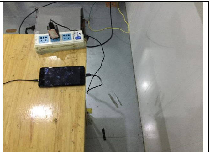
Conducted Emissions Test Setup Side View
