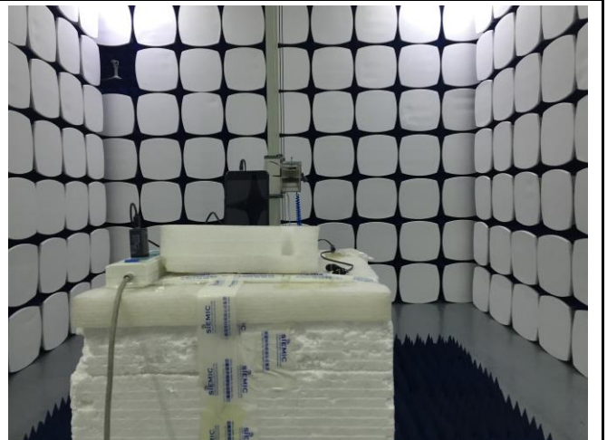
Radiated Spurious Emissions Test Setup Above 1GHz
