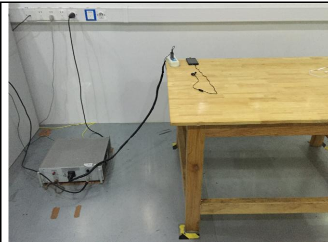
Conducted Emissions Test Setup Front View
