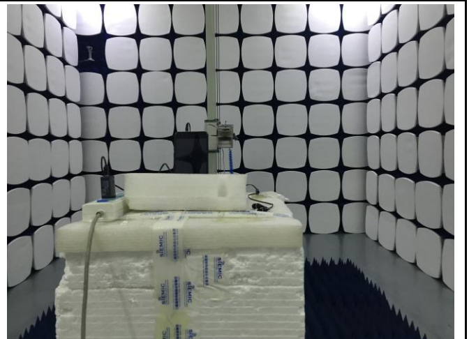
Radiated Spurious Emissions Test Setup Above 1GHz
