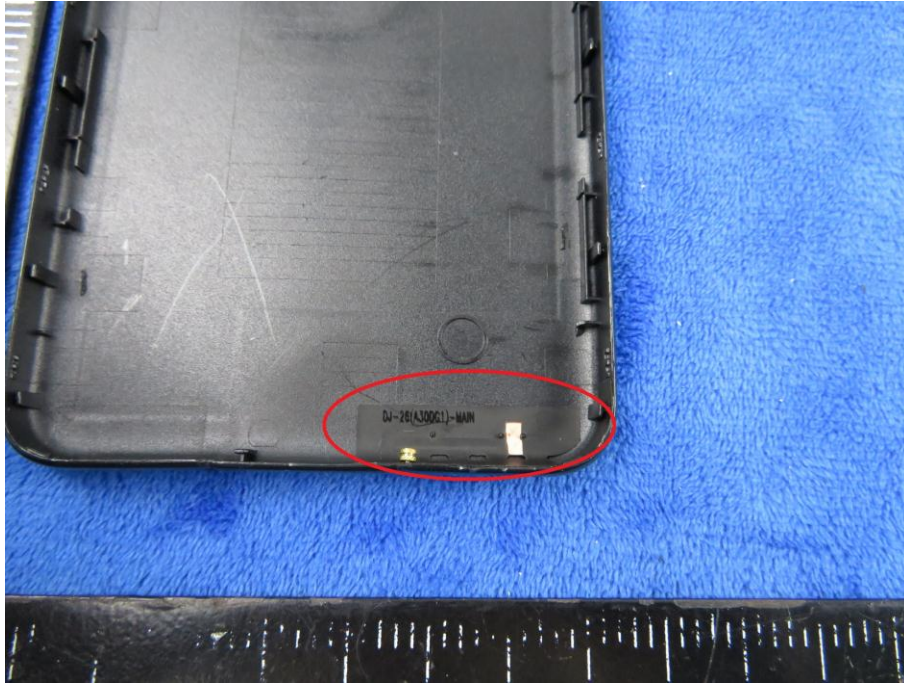
GSM/PCS/UMTS-FDD - Antenna View
