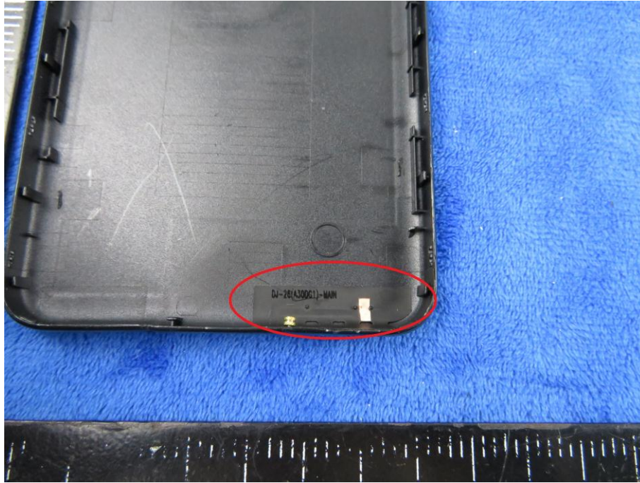
GSM/PCS/UMTS-FDD - Antenna View
