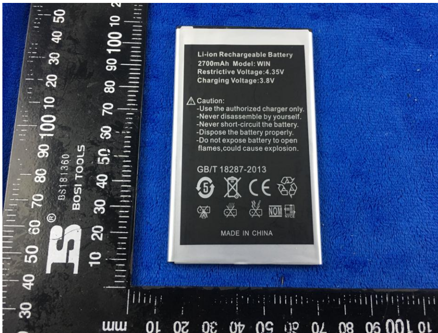
Battery - Rear View
